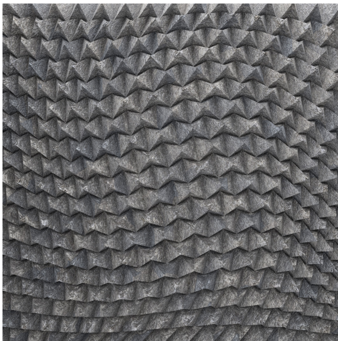
Feltfold: Rhino/Grasshopper generated panellisation of a waterbomb base across a surface of lofted curves.
