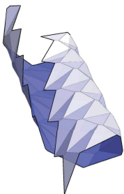
Figure 2. Two different states of folding of a Huffman grid (quadrilateral grid of identical degree-4 vertices).
