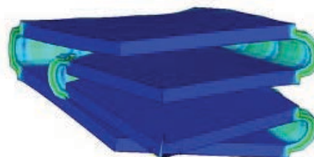
Figure 3. Finite element analysis results of scaffold self-folding driven by bilayer polymer actuators.
