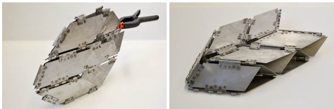
Figure 1. Single unit of a morphing panel (V2 mechanism), constructed from 1.0mm thick mild steel. Flat-folded, on left; deployed configuration, on right.
